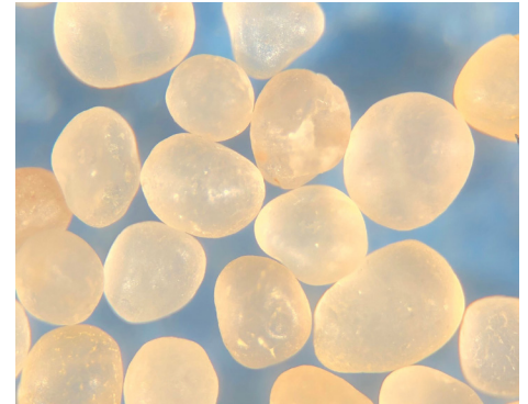
12/20-mesh premium frac sand has roundness and sphericity values typically greater than or equal to 0.8.
