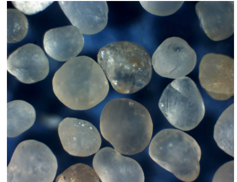
16/30-mesh premium frac sand has roundness and sphericity values typically greater than or equal to 0.7.
