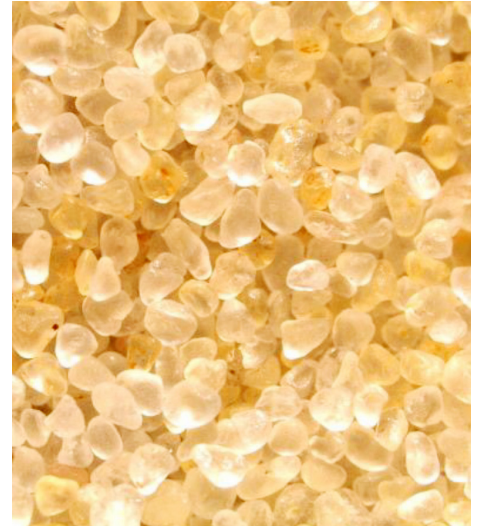
100-mesh premium frac sand has high silica content with roundness and sphericity values typically greater than or equal to 0.7.
