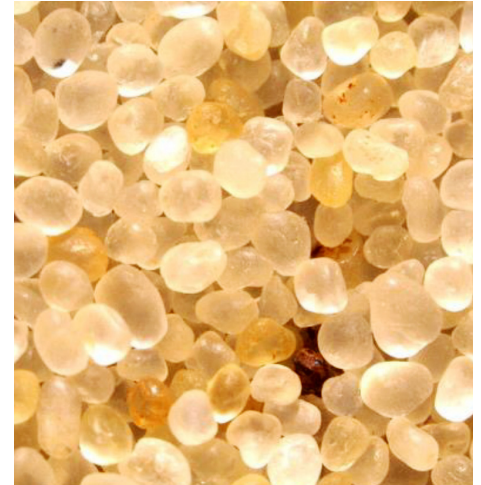
20/40-mesh premium frac sand has high silica content with roundness and sphericity values typically greater than or equal to 0.7.
